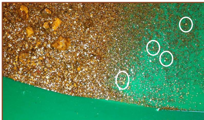
Figure 6. Crushed Iron pisolith sample containing gold grading up to 282 g/t in iron pisolites. (Source: TRP)
