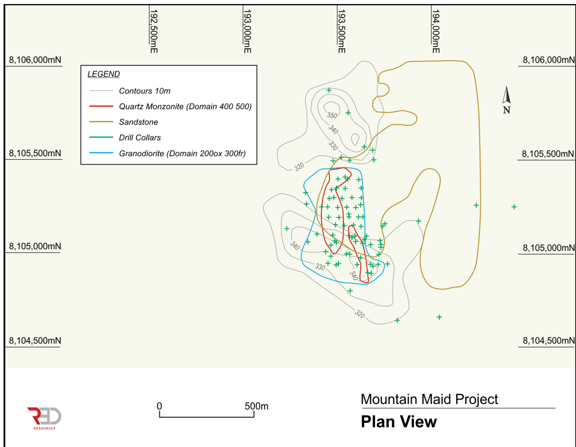
Figure 4. Plan view of the Mountain Maid resource including the location of drillhole collars and mineralised domains. Source: BMS.
