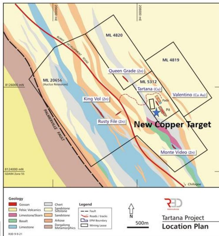
Figure 1. Tartana mining leases, the various prospects on the Tartana mining leases and neighbouring leases and the location of the new copper target. Note the New Copper Target is along strike from both Queen Grade and Monte Video zinc skarns. Note Monte Video or King Vol projects are not on the Tartana mining leases.
