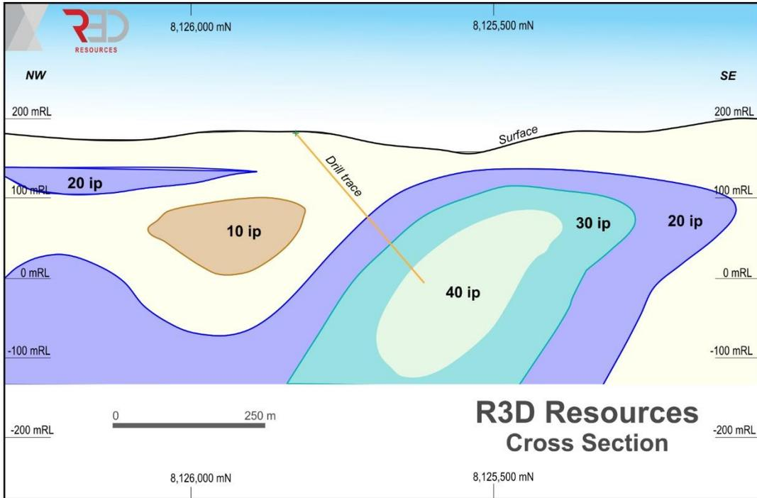
Figure 4. Proposed drillhole path and IP anomaly isopachs in cross-section.
