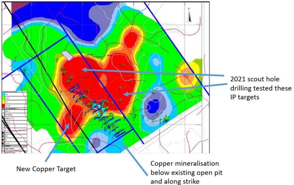
Figure 2. The New Copper Target in relation to the IP anomaly across the Tartana mining leases. The 2021 drilling programmed focused on IP anomalies east of the mineralisation in the open pit whereas the New Copper Target is to the west of the open pit mineralisation and potentially coincides with the northeast trending structural trend.
