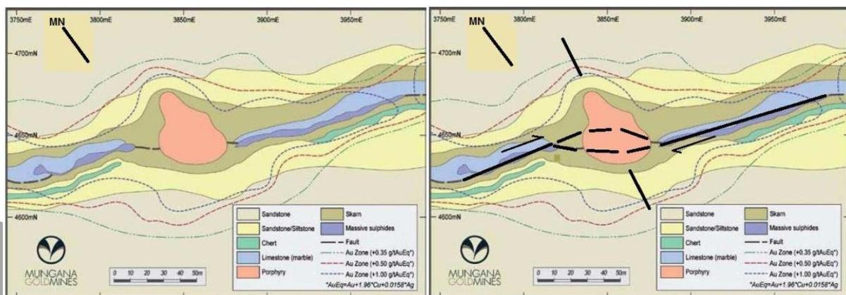
Figure 3. Mungana copper/gold porphyry model with zinc skarns (blue) emanating from the central porphyry (pink). From Nethery, J. 2015 Chillagoe District Mineralisation – A Tectonic Model. SMEG. Mines & Winds 2015
