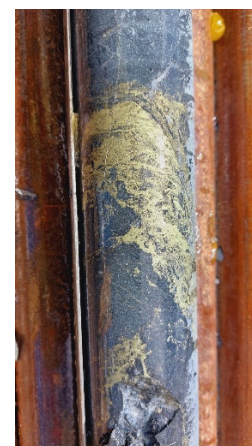
Figure 5. (a) Oxide, transitional and primary (fresh) resource estimation for the Tartana open pit using inverse distance estimation and a 0.2% Cu cutoff grade. (b) Primary copper mineralisation from drillhole D15.
