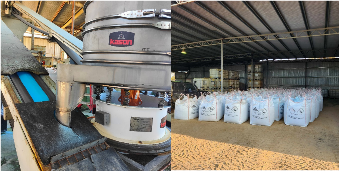
Figure 1. (a) Screening of copper sulphate pentahydrate prior to bagging. (b) copper sulphate pentahydrate bags ready for collection.
