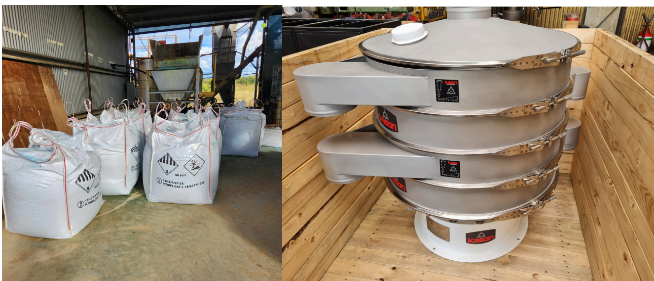
Figure 1. (Left) Production toward the second shipment. (Right) The new Kason Kason Vibroscreen Separator.
