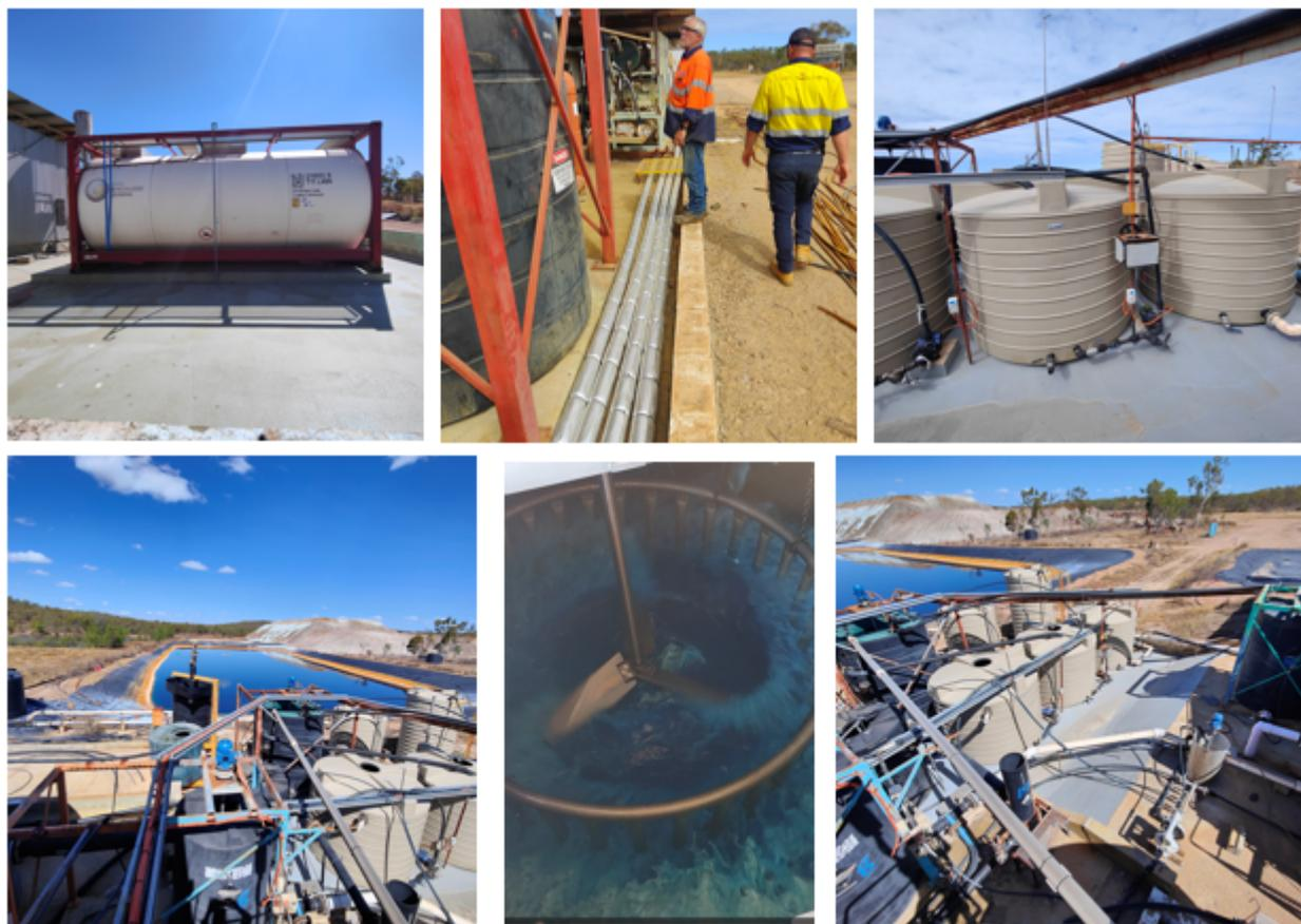
Figure 1. *Tartana Solvent Extraction – Crystallisation Plant. Clockwise – New acid tanks with delivered acid, Inspection of pipework, New tanks for copper stripping, View of plant tanks and pipework, Copper sulphate crystals in crystalliser, Plant, PLS pond and heaps for leaching in distance.*
