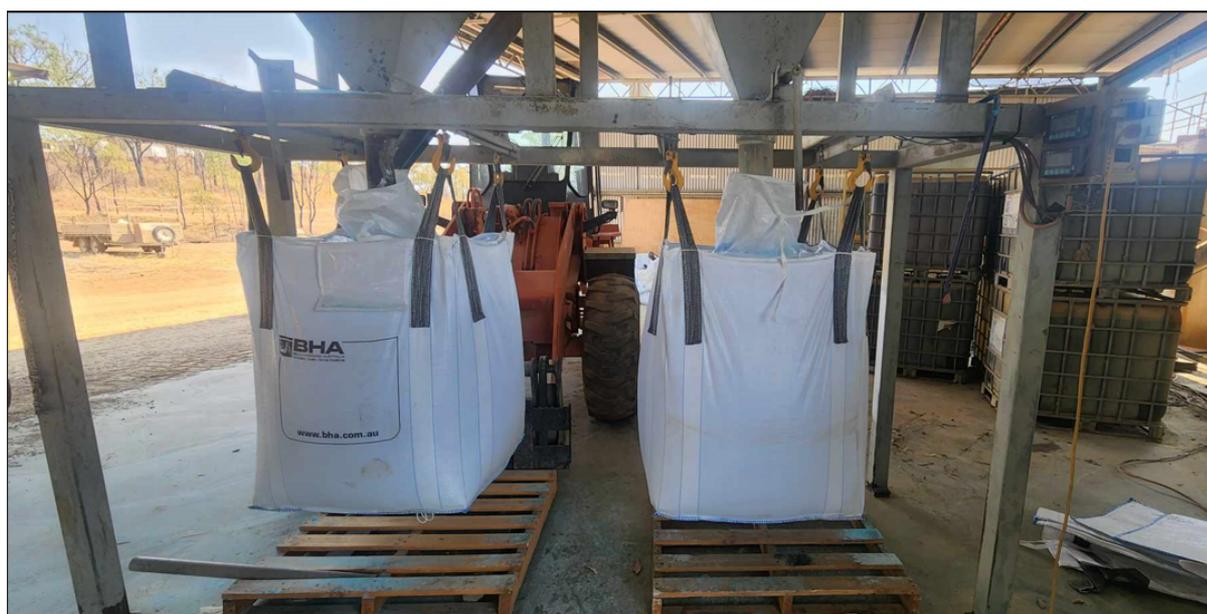
Figure 3. Loading of screened copper sulphate pentahydrate into bulka bags.
