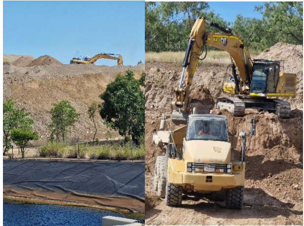
Images: Mining the open pit fill containing extractable copper and stacking the lower heap leach pad.
