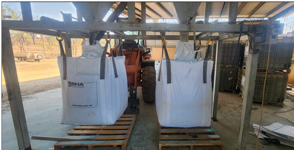
Figure 4. Loading bulka bags of copper sulphate pentahydrate after drying and screening.
