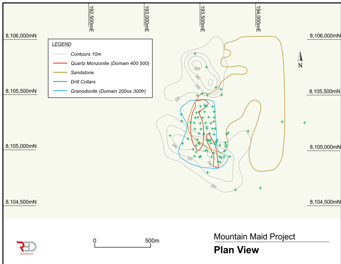
Figure 11. Plan view of the Mountain Maid resource including the location of drillhole collars and mineralised domains. Source: BMS.
