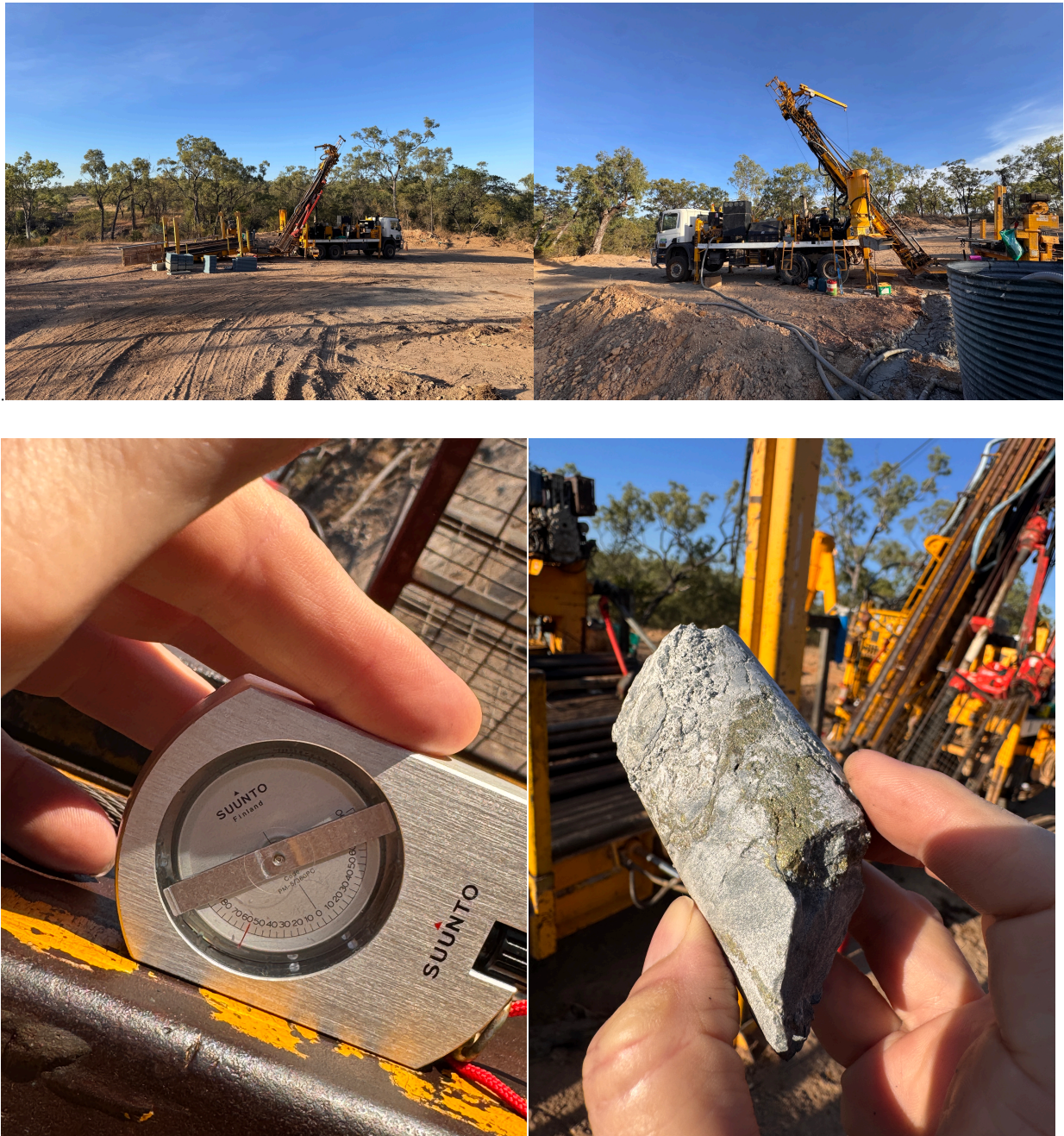
Figure 1. (a) and (b) UDR 650 rig drilling D10 Tartana copper project. (c) checking drillhole inclination (d) typical chalcopyrite (copper) mineralisation in core at 122.5m in D10 (Note: this is not representative of the entire hole and first assays for the interval 0-125.5m will be available in approximately four weeks. Note:
