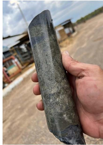
Figure 5 – Semi massive sulphide in drill core from RDD 002 at 590m.
