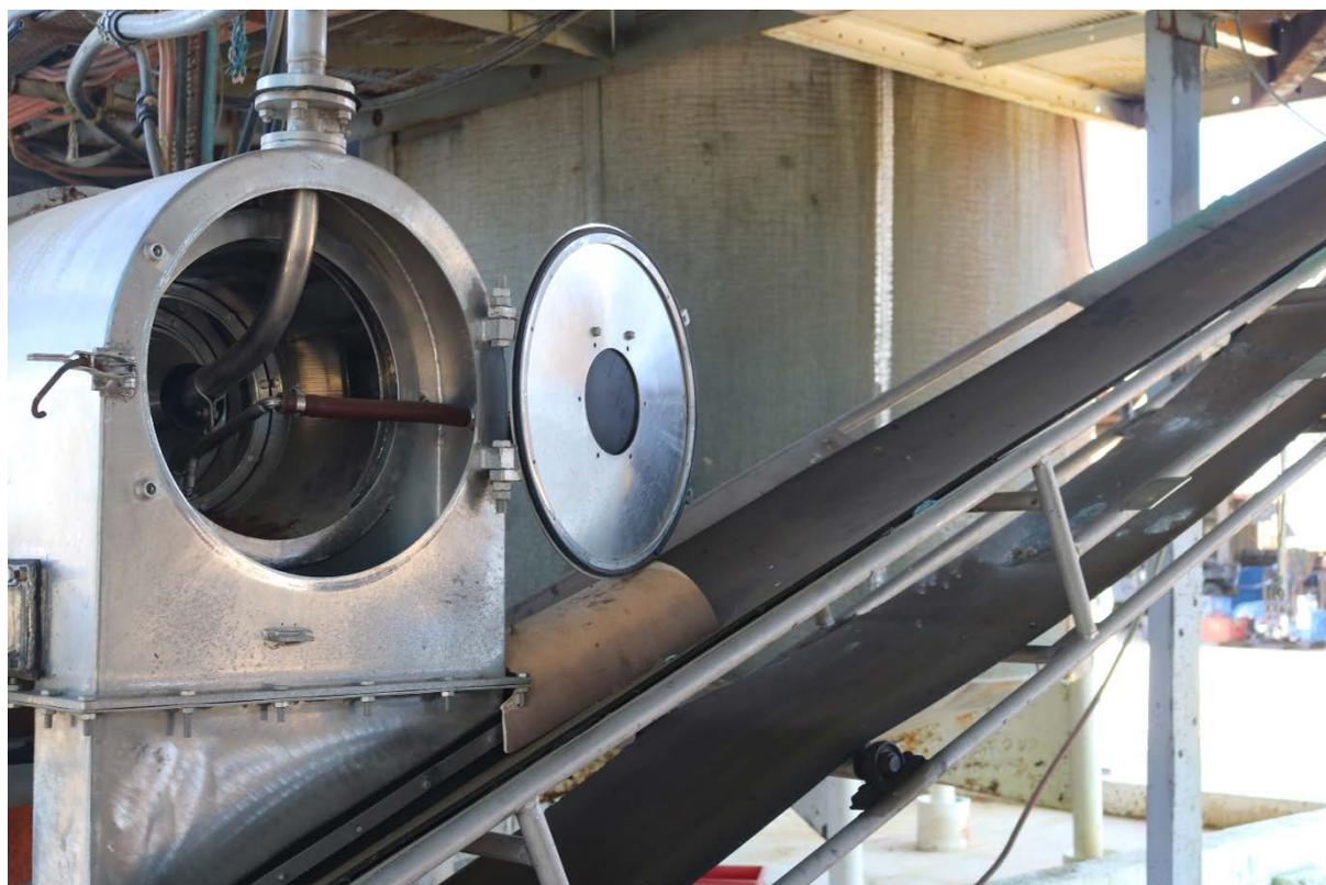
*Figure 8 – Centrifuge for crystallising copper sulphate.*
