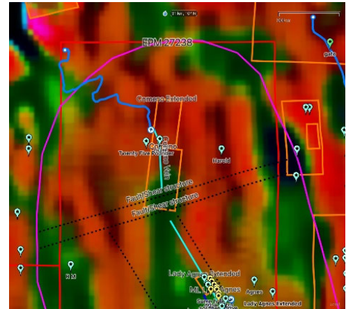
1vd-2vd-merge-RTP image showing mapped structures, Comeno vein and Lady Agnes vein (Magnetics from GeoResGlobe)
