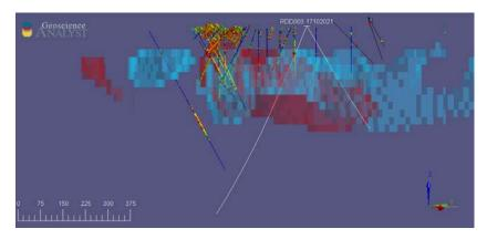
Figure 7 – Cross-section showing the drill paths of RDD002 and RDD003 and the position of historical drilling associated with open pit mineralisation.
