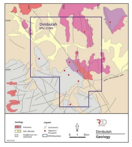
Figure 11 – Geology of the Dimbulah porphyry copper project area.
