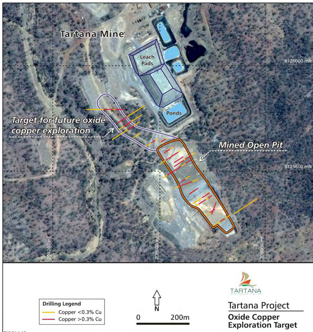
Figure 12: Plan of the Tartana project with detail of exploration target area immediately north of the existing open pit
