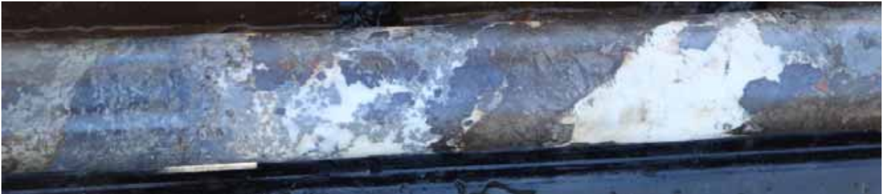
Figure 13 – Queen Grade drill core showing zinc, lead and iron sulphides and carbonate typical of skarn mineralisation in the Chillagoe region (9 December 2017).
