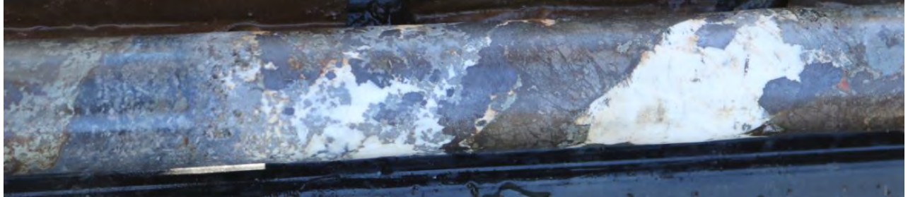
Figure 13 – Queen Grade drill core showing zinc, lead and iron sulphides and carbonate typical of skarn mineralisation in the Chillagoe region (9 December 2017).
