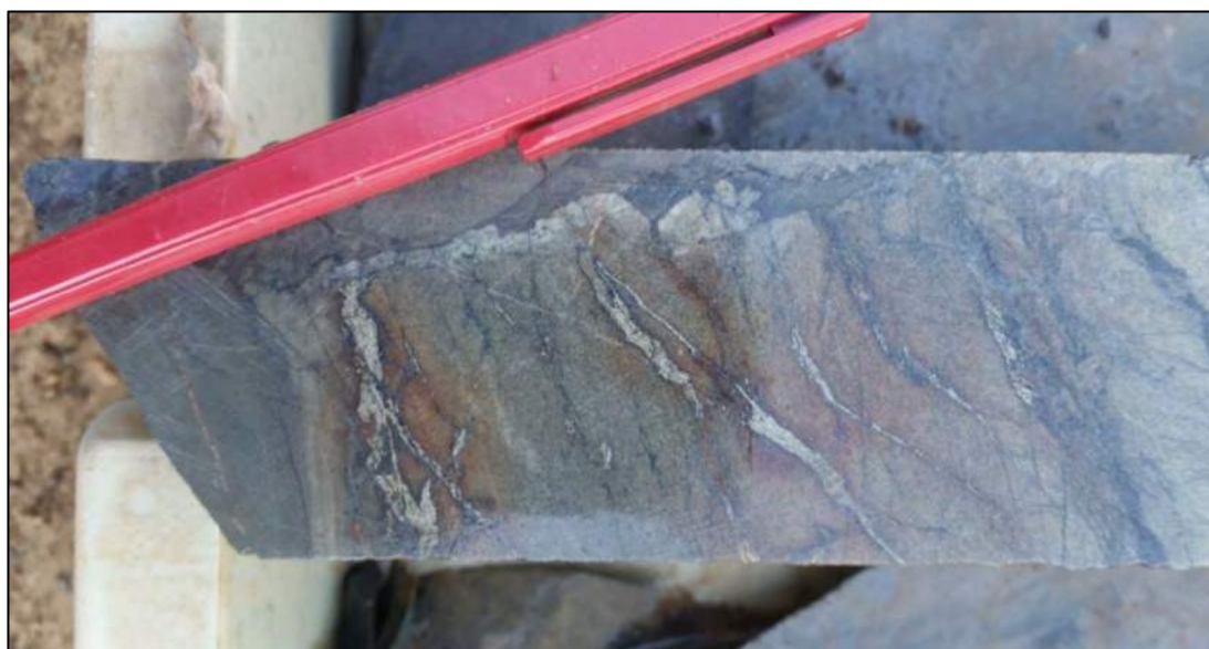
Figure 7: Half-core sample from TDH13 at 129 m showing pyrite veins with silica–carbonate (ankerite) alteration
